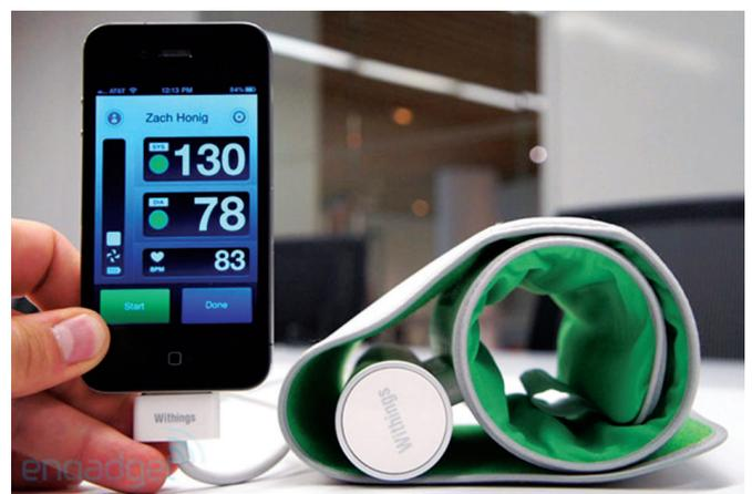
Figura 1. *Withings Blood Pressure Monitor* conectado ao *smartphone* (*Iphone*).
